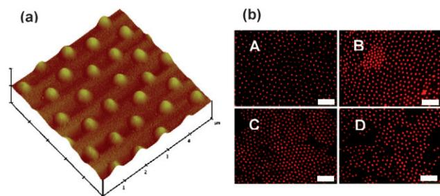
**Fig. 1** Surface imaging of the hydrogel nanoparticles (a) deposited from PBS solution *via* horizontal convective assembly at 37 °C on a mica surface and analyzed using AFM in air at 25 °C in tapping mode (see Experimental for details) (b) NPs deposited on glass slides by self-adsorption from PBS solution at 37 °C and analyzed using fluorescence microscopy. No particle aggregates were observed under the experimental conditions used. (a) Vertical scale bar = 100 nm, (b) Scale bars = 5 μm.
