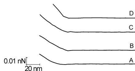
**Fig. 2** Characteristic force curves measured using AFM between a cantilever tip and one nanoparticle grafted on a mica surface for the NP batches listed in Table 1. The grafted NPs were immersed in PBS at 37 °C for 1 h prior to the experiment. The increase in the slope of the curve in the indentation regime (corresponding to the left part of the force curve) from batch A to batch D corresponds to an increase in Young modulus as described by the eqn (1).
